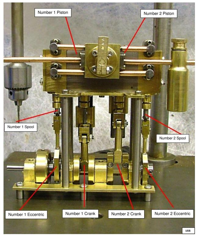
It is easier to set up if the top and bottom are not joined at the start, as it is easier to adjust the crankshaft timing, but can be done with things built up.
