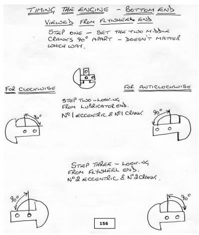
**<u>Step 1</u>**: To start, set the two cranks either side of the crankshaft centre bearing block at 90 degrees (or very close) to each other and tighten up. These will not be moved again.
