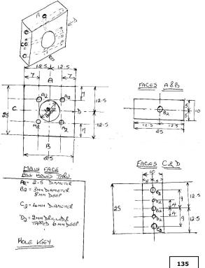
I had forgotten that I had a few pictures left in my camera, so I have decided to make a post out of these. The blocks need to be made and all completed before I could carry on anyway, because the bits that fit to it have to be lapped into the main bore and the soldering has to be done first just in case we get a little bit of distortion in the main bore. I suppose you could bore it after soldering but it might be a bit difficult to hold well enough.
