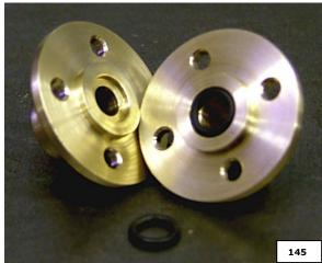
This o-ring stops steam leakage thru the control arm hole. The recess is bored 0.9mm deep (refer to Pic 145) to allow for an 0.1 mm crush on the o-ring.
