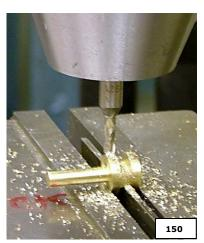
Refer to Pic 149. The slot is central on the spool depth. If you haven't got a 3mm cutter a 1/8" will suffice. Cut down to 3mm depth. Before you take out of the vice, scribe a line parallel to your cut across the face of the 4mm spigot; this is to show you where the control faces are after it is assembled in the block.
