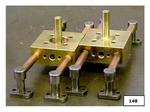
Put a bit of oil - I use multigrade or 3-in-1 (**Warning**: on no account use WD40 anywhere near this engine; it ruins certain types of o-ring seals!) and put the bits together and turn them. They should be silky smooth with no rock between the parts. If you've got rock, you've either been to the seaside or you have overlapped the parts. Make a new spool and start again! Don't worry about the bore; we make everything to fit that.
