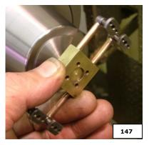
Refer to Pic 147. Being very careful about keeping your hands away from the chuck (I used my collet chuck because it is safer for me because I have to work left handed), gently feed the bore onto the rotating spool, get ready to let go just in case it galls up and starts spinning (galling is where the materials lock together; usually it is caused by the materials being the same or one is very soft).
