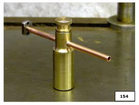
Pic 154 shows the bits silver soldered up. I soldered up the chamber and top first, then put it in the lathe to be cleaned up, then I soldered in the copper pipe. When soldering this in, make sure that the flange is in the up/down position otherwise you will have trouble filling the lubricator, but not emptying it. I put the hole on mine facing up, so if it does get blocked it can be cleaned out.
