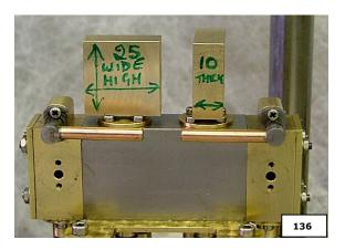
Pic 136 shows the size of blocks required. I have stated that these can be made out of brass or steel, preferably brass (a lot less hassle to drill and tap).
