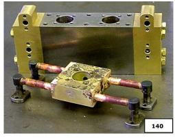
This now brings us to Pic 140. The block has been taken off the 'jig'. You can see that the flux has done its job keeping the soldered area clean, and because the heat was kept directly off the pipes, the joints on the flanges are totally untouched. The solder around the plugs has re-melted but they still have a good seal.
