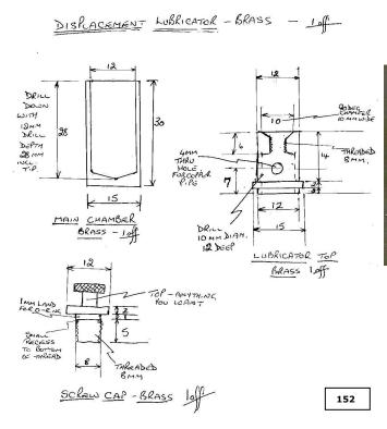
Three bits on the sketch (Pic 152); the fourth you have made previously - the longer of the two steam pipes.
