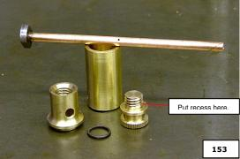
Pic 153 shows the three parts to be made, plus the long tube with a hole drilled half way along in line with the mounting bolt holes. The hole only goes in one side, mine is 0.7mm diameter, but you can use up to 1mm. If it under lubricates I can always open up the hole, but if it lets too much thru it is difficult to make smaller. The bit of text pointing to the cap is if the cap won't tighten down fully; just
