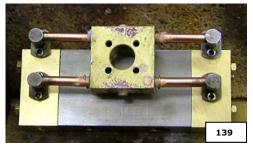
Pic 138 shows how to seal up the bit of the transfer holes that aren't required. I tapped the outside bit of the hole 4mm and screwed in a bit of brass threaded rod. You can just use a bit of rod if you want, or even make a feature of it by turning up a little cap with a spigot on it, your choice. I use screwed rod to stop it falling out in subsequent reheating. Don't block the steam transfer holes with the plugs.
