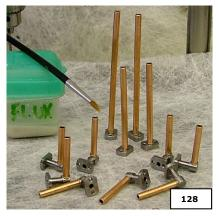
Onto Pic 128. On here I have assembled the parts and put one coil onto each joint. All that is left to do is paint a small amount of flux around the joint and stick some heat onto it. You will notice that I have protected my table because of the flux.
