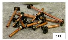
Now onto Pic 129. Here are the bits straight out of the quench. You will notice on the standoff ones especially the bright silver area on the steel and the clean area on the copper above the joint - this is the flux doing a great job.
