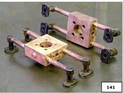
Notice all the good joints. I re-measured the main hole and there was no detectable deformation, so looks like we are in with a chance of making a good valve. Just got to wait until I can get the bits made.
