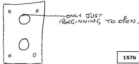
Slacken off nut at bottom of piston spool valve. Turn engine until piston is at TDC.
