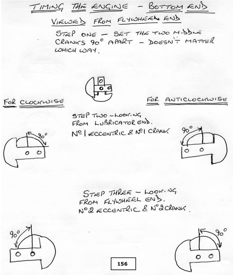
**Step 1:** To start, set the two cranks either side of the crankshaft centre bearing block at 90 degrees (or very close) to each other and tighten up. These will not be moved again.
