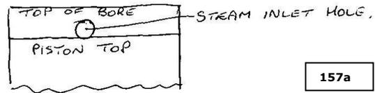
Slacken off nut on crosshead and screw the piston rod in the correct direction to bring the top of the piston in line with the bottom of the steam inlet hole. (See [Pic 157a](#))
