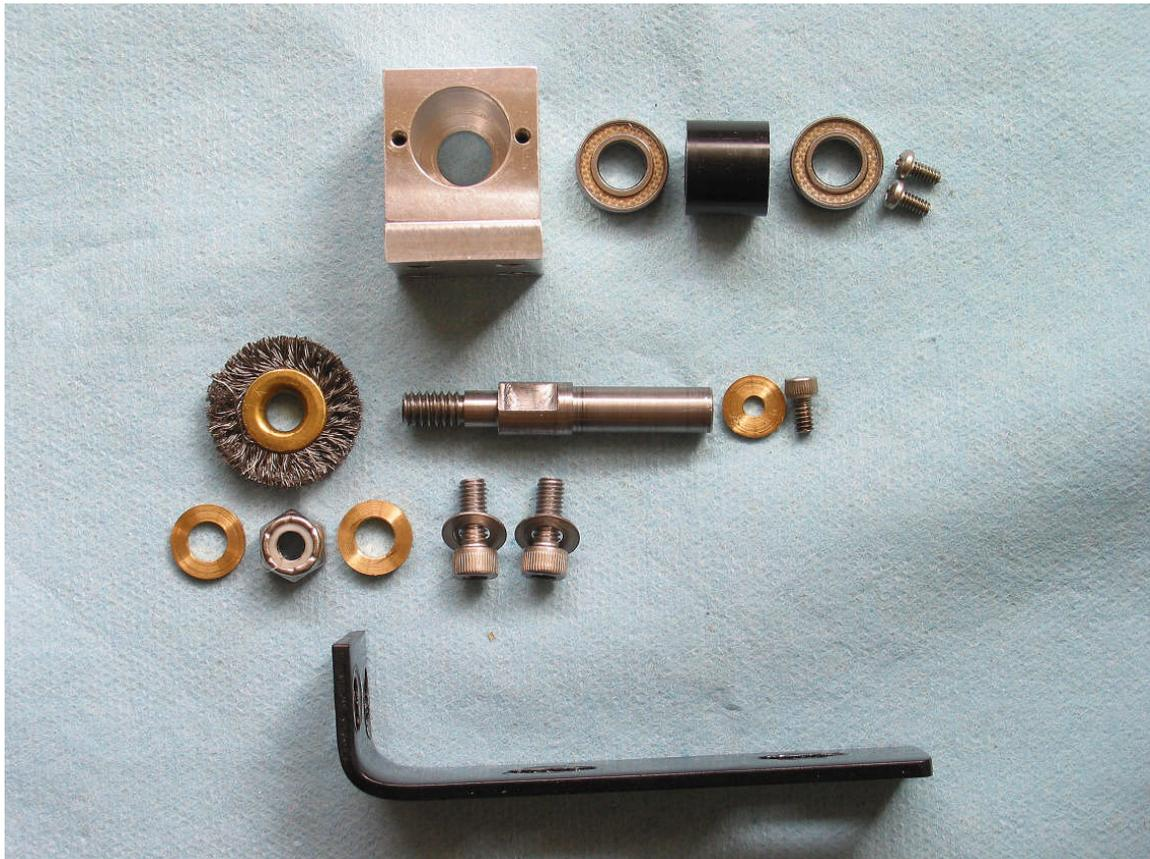
6. Now make the mounting bracket. As your saw may differ from mine you will need to determine how to mount the brush. Try to leave enough vertical and lateral adjustment to position the brush so that the center of the brush aligns with the center of the thrust bearing, and some rotational adjustment so the brush can run in line with the blade.
