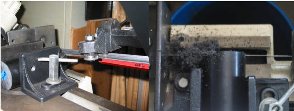
*Delrin is the messiest stuff to cut. In these shots the blade is running, with very few chips on the upside of the stock.*
